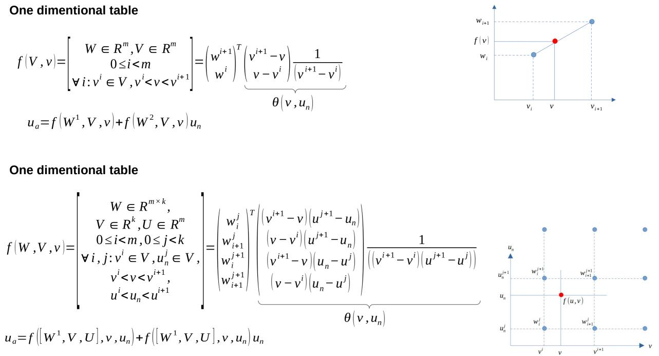
Table adaptive control relies on linear or bilinear interpolation from tables, with coefficients that are adjusted adaptively according to MRAC control law. The following graphs illustrate the simulation of vehicle speed tracking, taking into account the effects of tire characteristics and the nonlinear behavior of the engine. The method is based on the assumption that the system's characteristics vary at different speeds and with different levels of throttle and brake pedal engagement.
