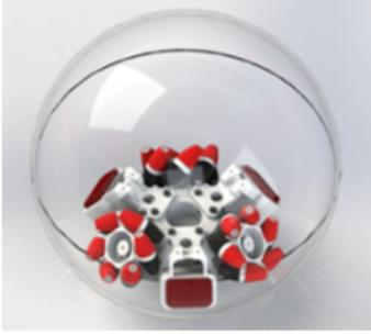
Fig. 1. Spherical robot with an internal platform having three mecanum wheels [11].
