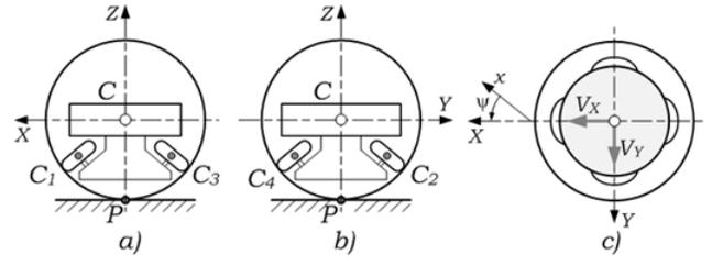
Fig. 2. Kinematic scheme of the spherical robot with an internal platform having four omni-wheels: a) side view; b) front view; c) top view
