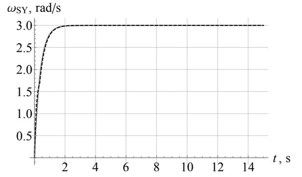
Fig. 4. Dependence  $\omega_{SY}$  obtained from the results of modeling equations (13) (gray solid line) and equations (10) (black dashed line) with control torques calculated at low program speed.
