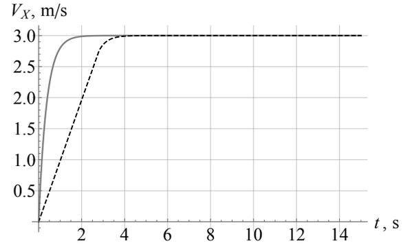
Fig. 5. Dependence  $V_X$  obtained from the results of modeling equations (13) (gray solid line) and equations (10) (black dashed line) with control torques calculated at high program speed.
