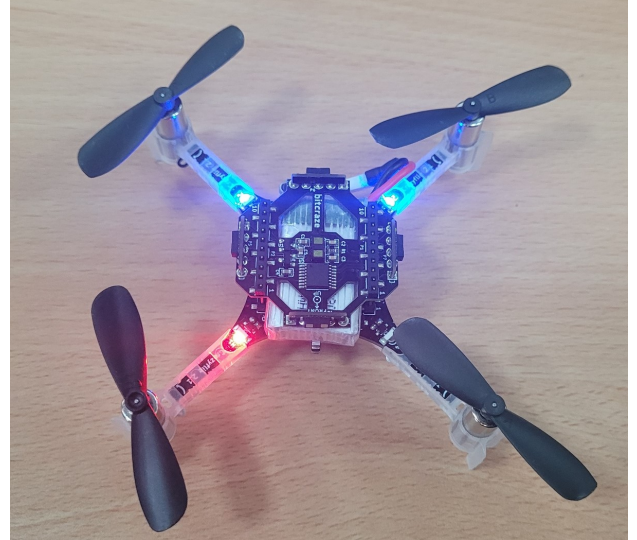
Fig. 1. Crazyflie 2.1 Nano quadcopter with Multiranger distance measurement deck
