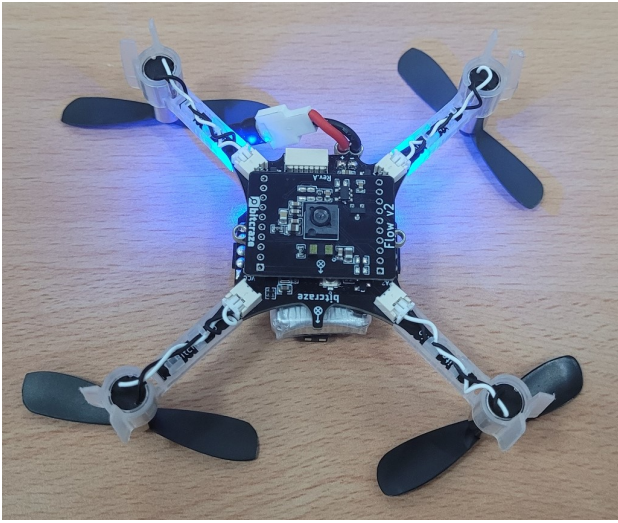
Fig. 2. Crazyflie 2.1 Nano quadcopter with Optical Navigation Flowdeck V2
